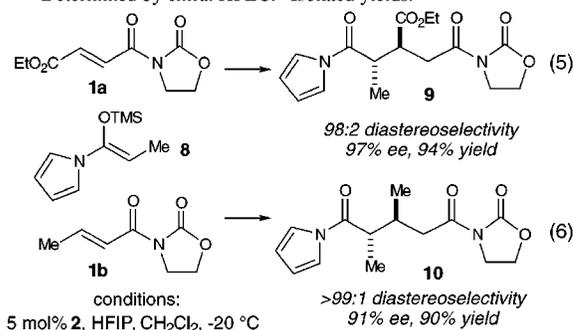
example, the stereoselectivity of the addition process is generally improved with increasing enolsilane alkyl substituent size. Reactions of methyl thioester enolsilanes were complete in less than 12 h at –78 °C or within several hours at –20 °C. (*Z*)-Substituted aryl ketone enolsilanes afford high yields of the requisite adducts in less than 60 min at 0 °C.
